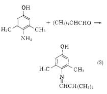
The base was treated with a slight molar excess of *n*-butyraldehyde in methanol solution containing 5% palladium on charcoal catalyst, and hydro-
