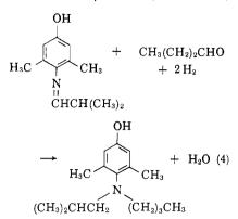
tion was poured over crushed ice. The tan, crude 4-(n-butylisobutylamino)-3,5xylenol was recrystallized twice from pentane to give white needles (melting point, 89-90° C.).
